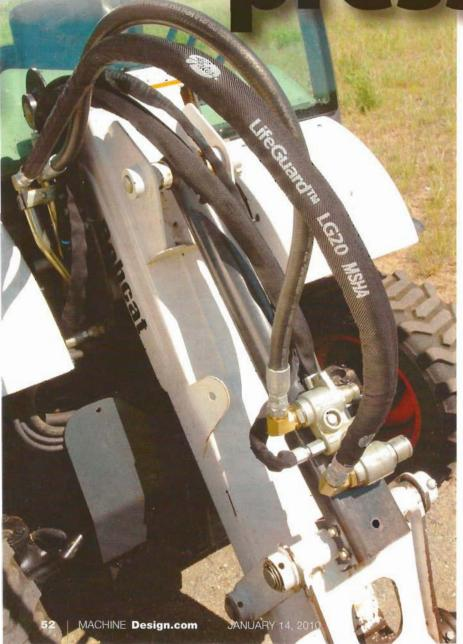
Modern hydraulic hoses vary widely in terms of pressure ratings, temperature ranges, and materials, but all consist of three basic components: tube, reinforcement, and cover.
